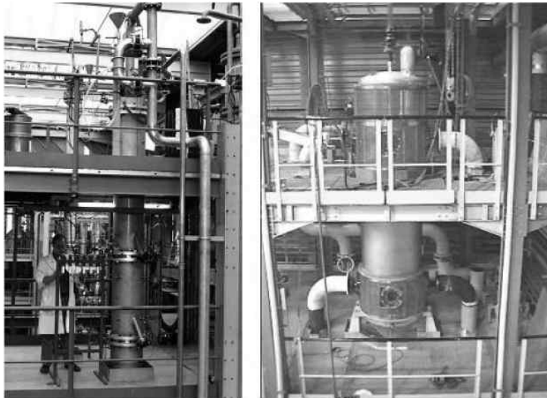
Figure 5.11. Examples of mock-ups used to study reactors using heterogeneous catalysts: fixed bed (left) and moving bed (right) © IFPEN, © P. Chevrolat
